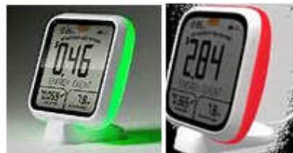
American company Ambient Device's – Ambient Home Joule changes colour to indicate when energy prices are high (red), medium and low (green). 34
