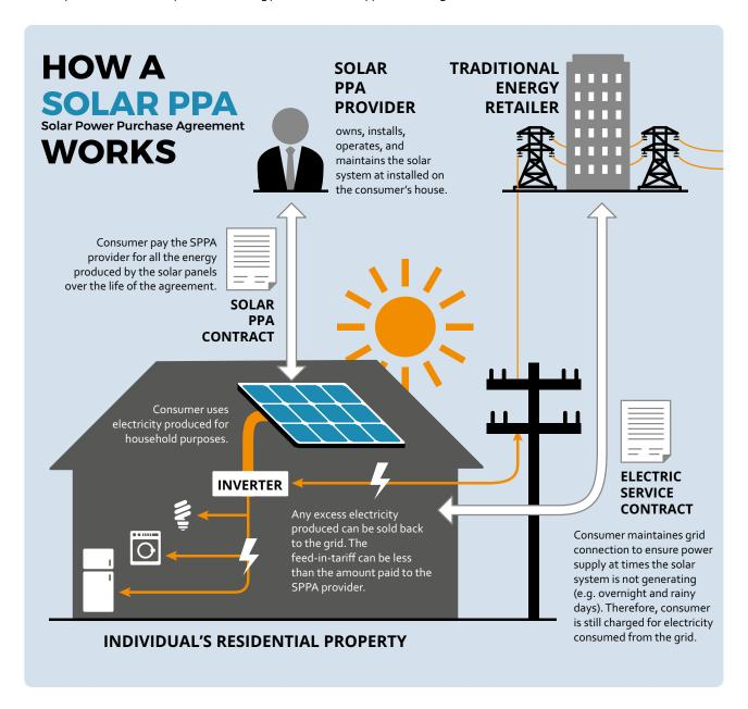
The purpose of solar PPA is to reduce the household's energy costs by reducing the amount of electricity they buy from traditional energy retailers. But, as we see with case study 7, a poorly structured solar PPA can have the opposite effect.
